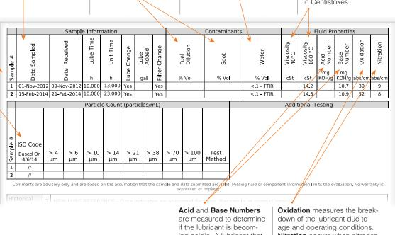
are measured to determine if the lubricant is becoming acidic. A lubricant that becomes too acidic can cause corrosion to internal engine components. Note that acid and base numbers do not begin at zero. Oxidation measures the breakdown of the lubricant due to age and operating conditions. Nitration occurs when nitrogen oxides react with the lubricant, causing deposit formation and an increase in viscosity. Note that oxidation and nitration readings do not begin at zero.
